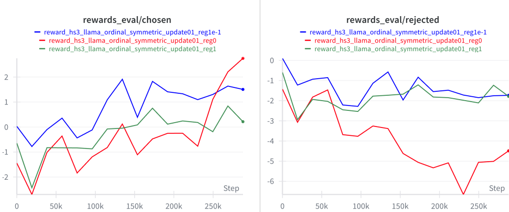
Figure 4: Evaluation reward values for chosen (left) and rejected (right) responses across different regularization settings. Without regularization (red), both chosen and rejected rewards diverge to extreme values. With regularization (blue and green), both reward types remain bounded and stable.
